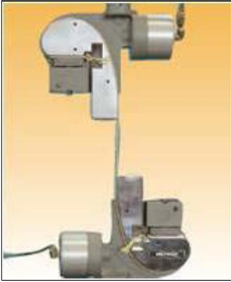
Fatigue tests on metals can be performed using a variety of pre-load mechanical and hydraulic grips.
