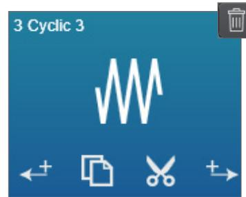
Key step controls - insert, cut, copy, paste and delete - are located within the step, reducing the amount of time putting steps together as compared to a traditional menu or toolbar-driven design
